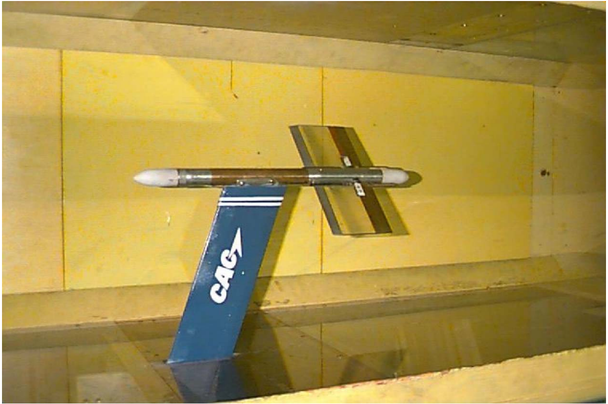
Fig. 2. Photograph of the aeroelastic model in the wind tunnel.
